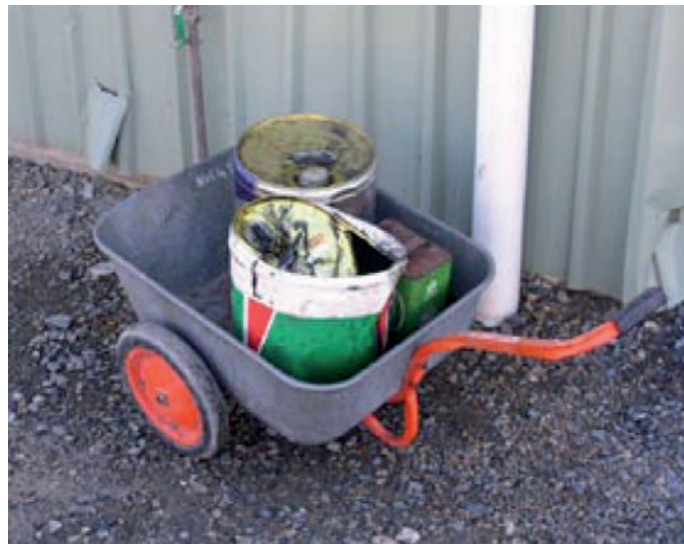
Above: Used oil stored in containers for long periods of time can create a fire hazard or develop oil leaks.
